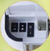
On/Off switch for heating element Variable speed Main switch
