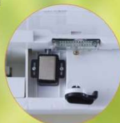
light for sensor Water level sensor
